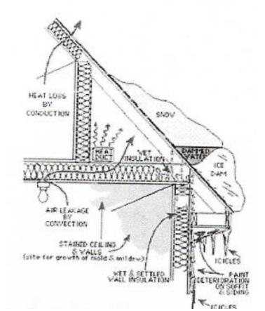
The diagram above shows the formation of a typical ice dam.
